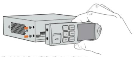
When installing the Teranex Mini Smart Panel to your Blackmagic Web Presenter, holding the panel with your fingers and thumb aligned with the panel's rear connector will help guide it into place
