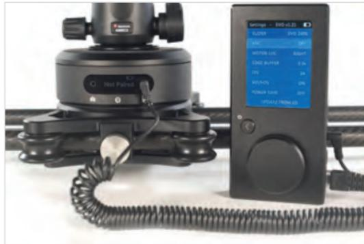
**Step 4.** Navigate to SETTINGS in the Rhino Motion Controller. Under "Arc", set it to "ON". The screen on Rhino Arc should now display "Paired". If it doesn't, make sure your cable is plugged in all the way and toggle the ON/OFF setting again.
